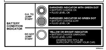
To determine the battery charge, check the battery test indicator (if equipped) on top of the battery. Refer to the illustration.
